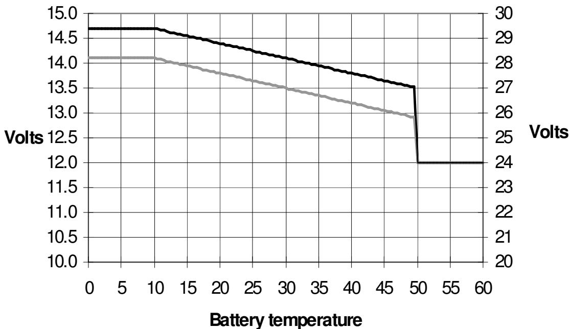
Default output voltages for Float and Absorption are at 25°C.
